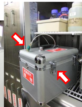
Locked and Anchored
